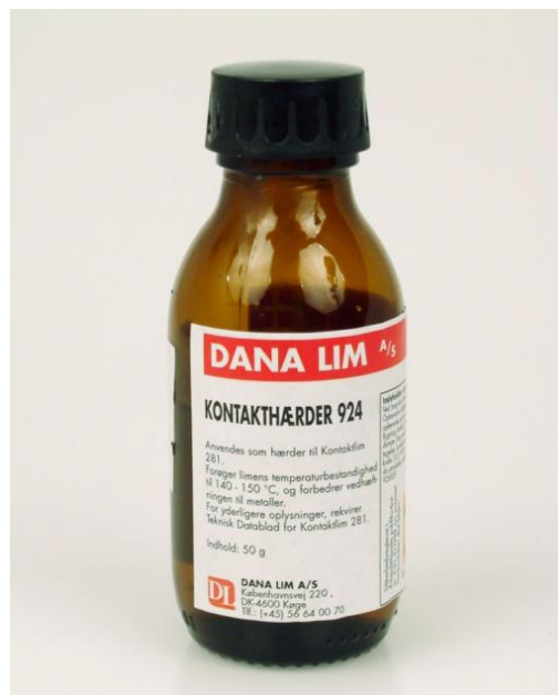
Contact Hardener 924 is added to contact adhesive 281 & transparent contact adhesive 284 to increase heat resistance up to 150 °C (depends on strength requirements)
